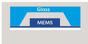
WLC module (wafer level glass capping)
