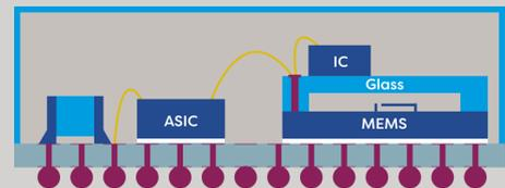
WLC: Wafer level capping (glass lid) in a SiP- application
