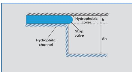
**Capillary stop valve cross-section**
